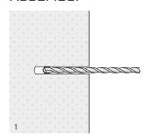
Drill a hole in rotary percussion mode
