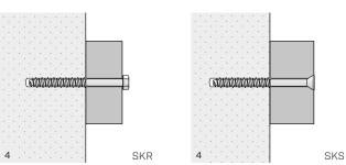
Ensure the anchor head is in complete contact with the object to be fixed
