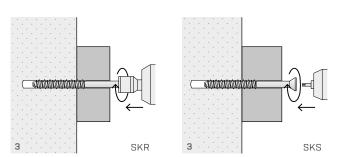
Position the object to be fixed and install the screw with a pulse screw gun
