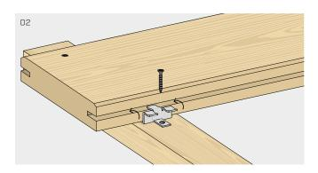
Insert the GAP3 fastener into the groove cut so that the clip's central tab adheres to the groove in the board.
