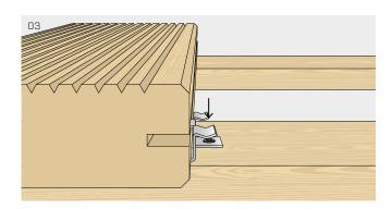
Fix the screw in the central hole.
