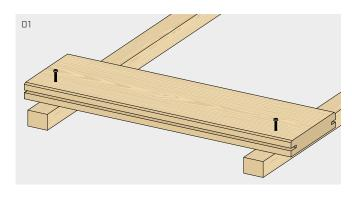
First board: fix it with suitable screws, left visible or hidden thanks to specific accessories.
