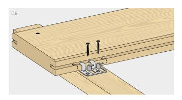
Insert the GAP4 fastener into the groove cut so that the clips' central tab adheres to the groove in the board.
