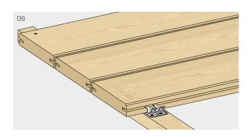
Repeat the operations for the remaining boards. Last board: repeat step 01.
