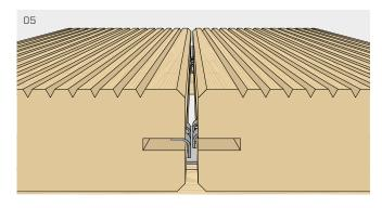
Using the CRAB MINI clamp, tighten the two boards until the gap between them is 0.16 - 0.20 inch depending on aesthetic requirements (see product page 424).
