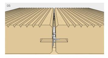
Using the CRAB MINI clamp, tighten the two boards until the gap between them is 0.12 - 0.16 inch depending on aesthetic requirements (see product page 424).
