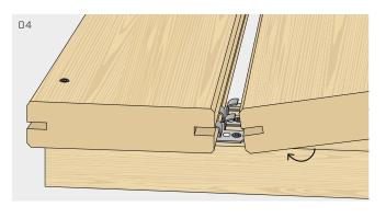
Position the next board by inserting it into the GAP4 fastener so that the two tabs adhere to the groove in the board.
