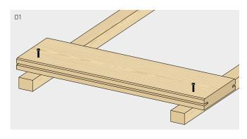
First board: fix it with suitable screws, left visible or hidden thanks to specific accessories.
