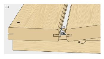
Position the next board by inserting it into the GAP3 fastener so that the two tabs adhere to the groove in the board.
