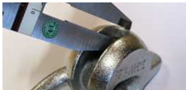
Method to measure minimum shank thickness m_{\min}
