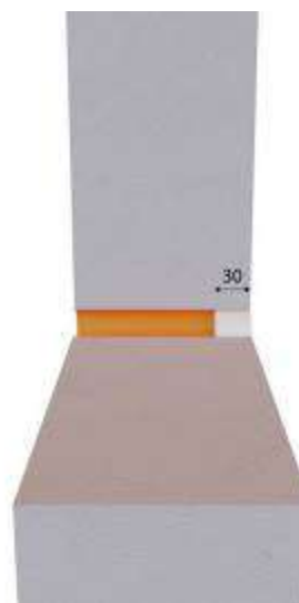
Figure A.1.2: Seal of a PVC pipe in a rigid wall.
