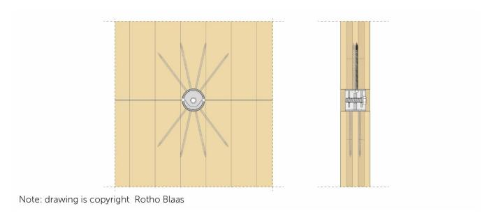
Page 26 of 28 of European Technical Assessment no. ETA- 24/0062, issued on 2024-06-26 Spaced connection single fasteners (example 1 RADIAL90+RADIALKIT90):
