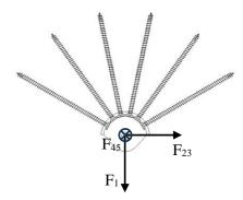
RADIAL connectors are intended for use for connections subject to static or quasi static loading. This includes seismic actions.
