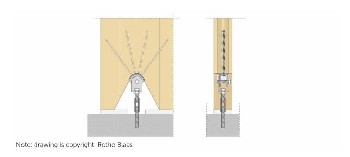
Timber-to-concrete or steel direct connection (example RADIAL90+BRACKET):
