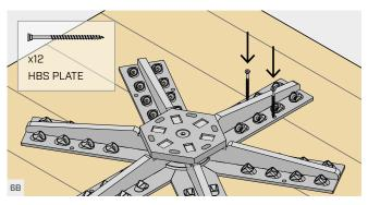
After inserting the hexagonal disc and countersunk head screw, insert 12 HBSP8120 screws into the 12 vertical holes provided in the 6 arms. These screws will hold the arms in place in the following phases.
