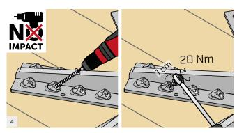
With a NON-PULSE screwdriver, insert the 48 VGS Ø9 screws inside the inclined washers, respecting the 45° insertion angle (use the JIGVGU945 pre-drilling template). Tighten by stopping about 1 cm from the washer and complete the screwing using a torque wrench by applying an insertion torque of 20 Nm.
