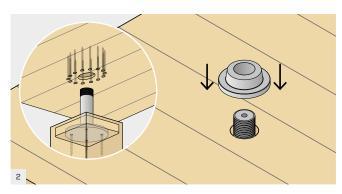
Fit the pre-drilled CLT panel with a circular hole of  $D_{\text{CLT}}$  diameter onto the cylinder. A compression reinforcement can be fitted to the bottom of the panel to increase strength. Screw the cone to the cylinder until it makes contact with the surface of the CLT panel.
