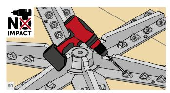
With a NON-PULSE screwdriver, insert the 12 VGS Ø9 screws inside the inclined washers closest to the cylinder, respecting the 45° insertion angle (use the JIGVGU945 pre-drilling template). Screw it in stopping about 1 cm from the washer.
