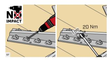
With a NON-PULSE screwdriver, insert the remaining 36 VGS  $\emptyset$ 9 screws inside the inclined washers, respecting the 45° insertion angle (use the JIGVGU945 pre-drilling template). Tighten by stopping about 1 cm from the washer and complete the screwing using a torque wrench by applying an insertion torque of 20 Nm.
