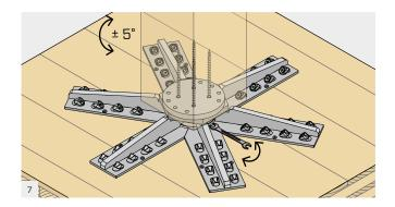
The slotted holes in the hexagonal disc allow the column to be rotated  $\pm 5^{\circ}$ . Turn the column to the correct position and tighten the 4 SPBOLT1235 bolts or MUT hex nuts of the SPRODS using a side wrench.
