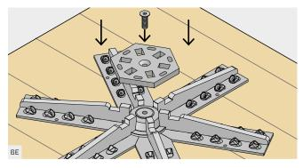
Insert the hexagonal disc and secure the countersunk head screw with a 10 or 12 mm male hexagonal wrench.
