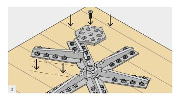
Place the 6 arms on the top surface of the CLT panel and cone. Insert the hexagonal disc in order to fit the 6 arms and fasten the countersunk head screw with a 10 or 12 mm male hexagonal wrench.
