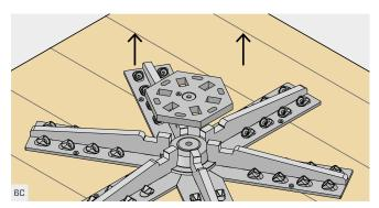
Unscrew the countersunk head screw and remove the hexagonal disc.
