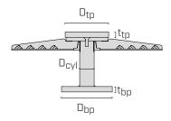
The code consists of the respective CLT panel thickness in mm (XXX =  $t_{CLT}$ ). SPI80MXXX for CLT panels with XXX =  $t_{CLT}$  = 200 mm : code SPI80M200.
