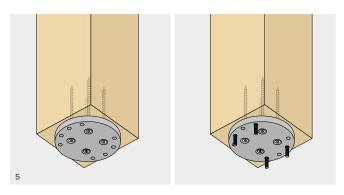
Fasten the upper plate to the lower face of the column using the VGS  $\varnothing 11$  screws, in accordance with the relevant installation instructions. The top plate is equipped with suitable threaded holes for fastening to the hexagonal disc. If SPRODS are used, after positioning the plate on the upper column, they must be screwed in, taking care to mark the minimum pull-through length in the upper plate.
