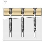
Adjust the other screws in a similar manner to level the structure.
