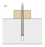
Drill the elements with a  $d_V$ = 8,0 mm diameter.
