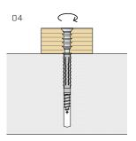
Attach the batten, screwing in the screw so that the head is flush with the timber.
