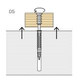
Loosen the screw based on the desired distance.
